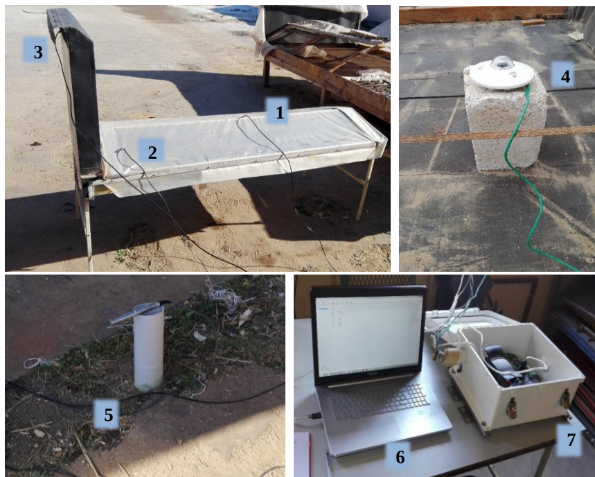
Figure 3.8 Experimental set-up of the solar tunnel dryer and the equipment.
