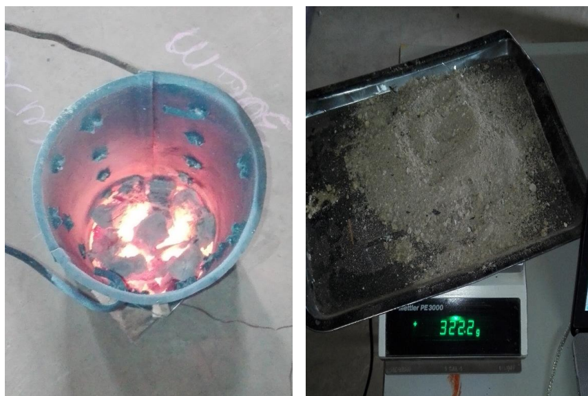
Figure 3.15 The DC of PLB after the smoke was released and the final product which is the ash
