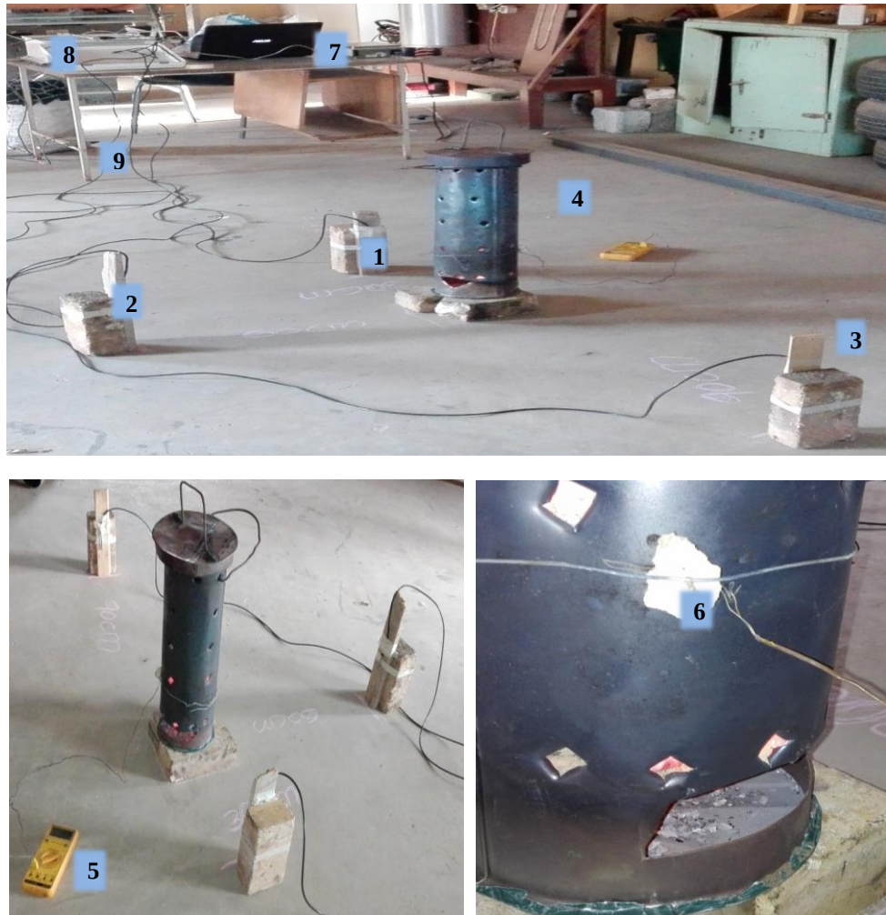
Figure 3.14 The side and top view of the experimental set up for the DC process throughout the experiment for all ages of PLB and charcoal
