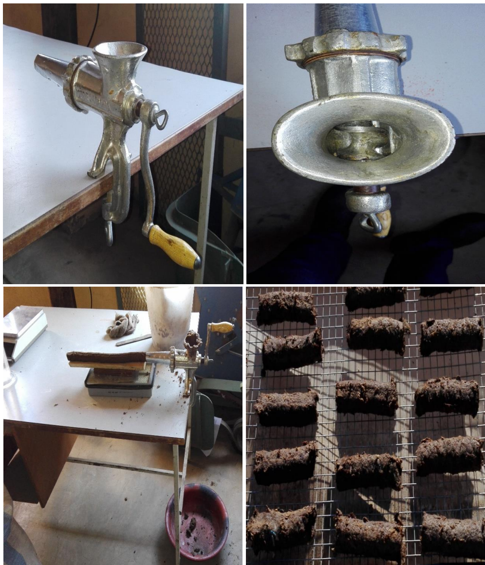
Figure 3.5 The hand grinder which was used to densify PL to make PLB
