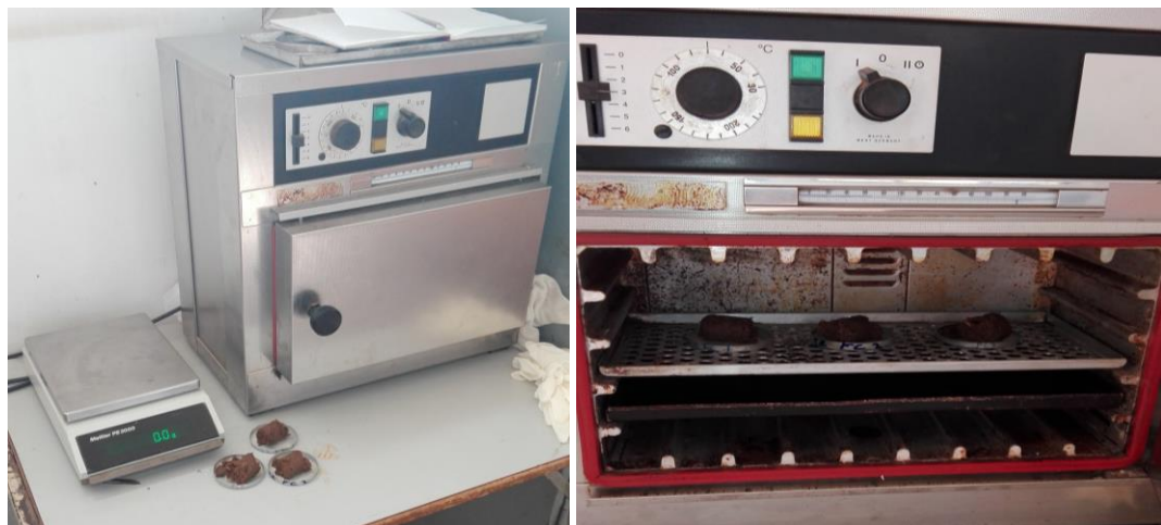
Figure 3.6 The instruments which were used for the moisture content determination.
