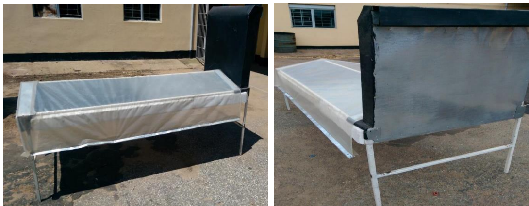
Figure 3.7 The side and rear views of the solar tunnel dryer
