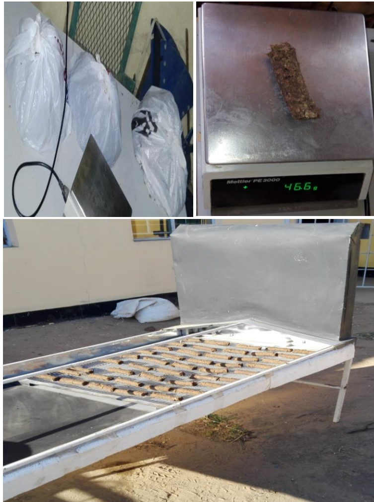
Figure 3.9 How PLB were stored (in plastic bags), weighed and how they were placed in the STD for the process of drying.
