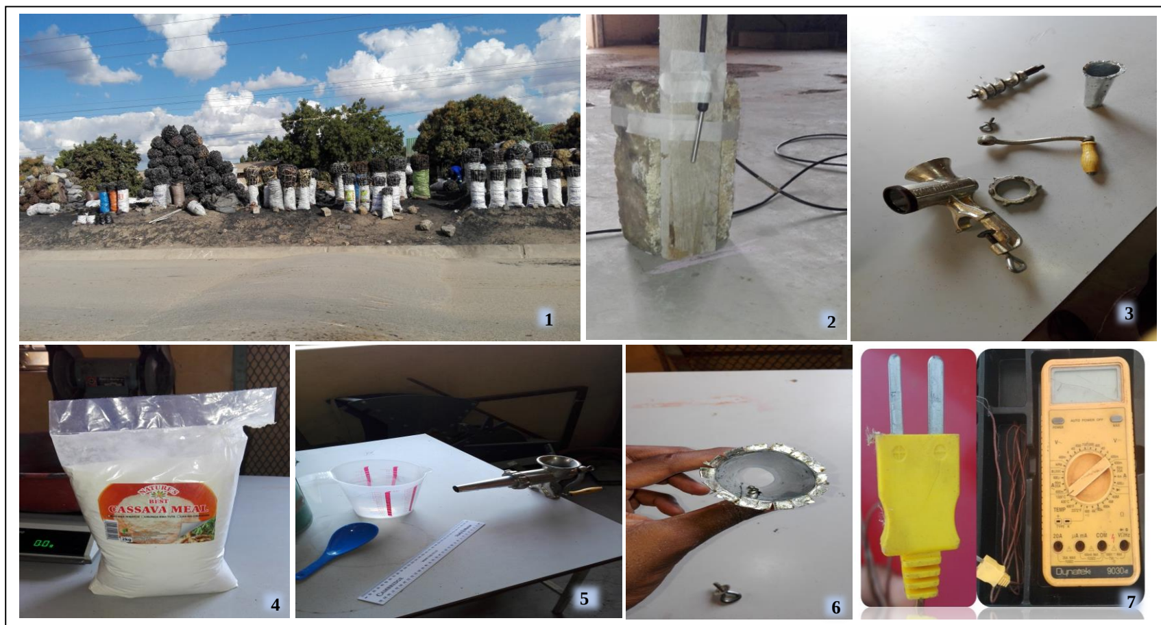
1=Charcoal, 2=Temperature probe, 3=Parts of a hand grinder (mincer mincer), 4=Cassava meal, 5=Measuring jug, ruler and spoon, 6=Nozzle and 7=Digital multimeter with Type k Temperature probe.
