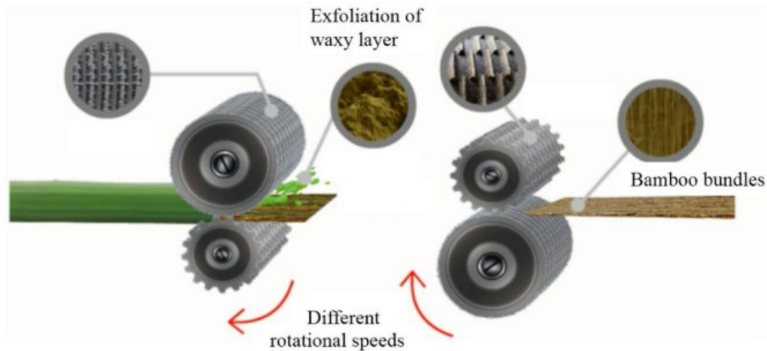
Figure 2.3: Diagrammatic Representation of the innovative fluffer machine invented by the Chinese Academy of Forestry. Extracted from Huang et al. (2019).
