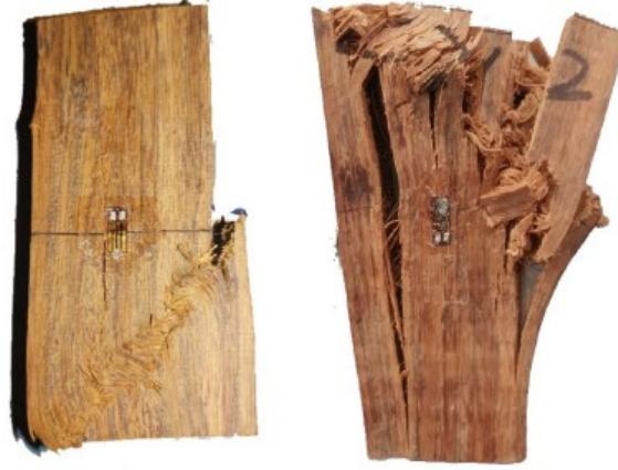
Figure 2.5: Critical failure mechanisms in compressive bamboo Scrimber samples. Extracted from Wei et al. (2020).
