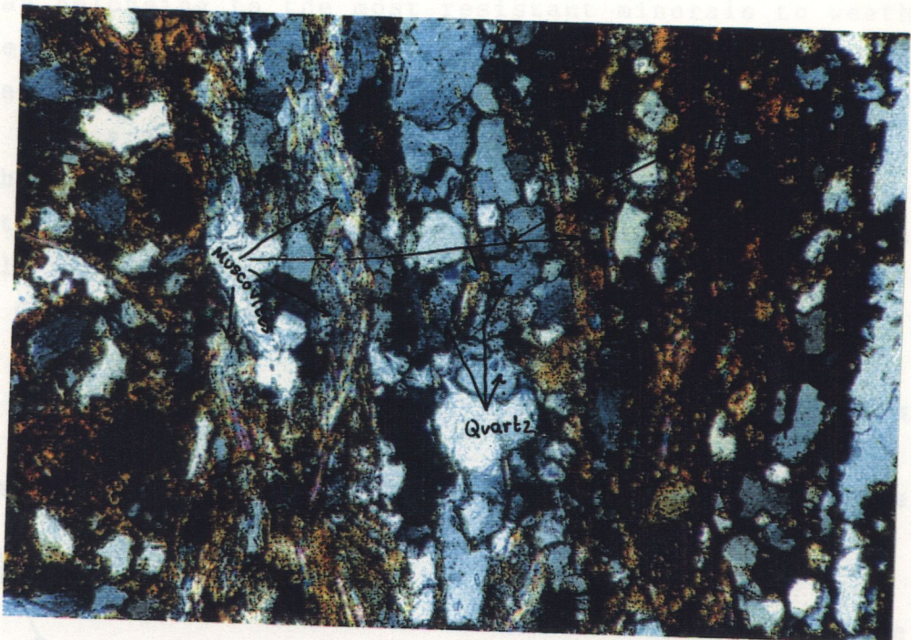
Photo 5: Rock fragment containing muscovite and quartz, showing parallel arrangement of minerals, typical of metamorphic rocks. (E horizon Profile 3, 30-35cm) Magnification: 6.3x 1.25 (PPL)
