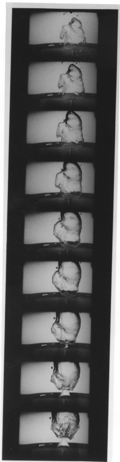
Plate 1(a) Lateral Spreading of Bubble at 20.38 l/min. d_0 = 3.0 mm
