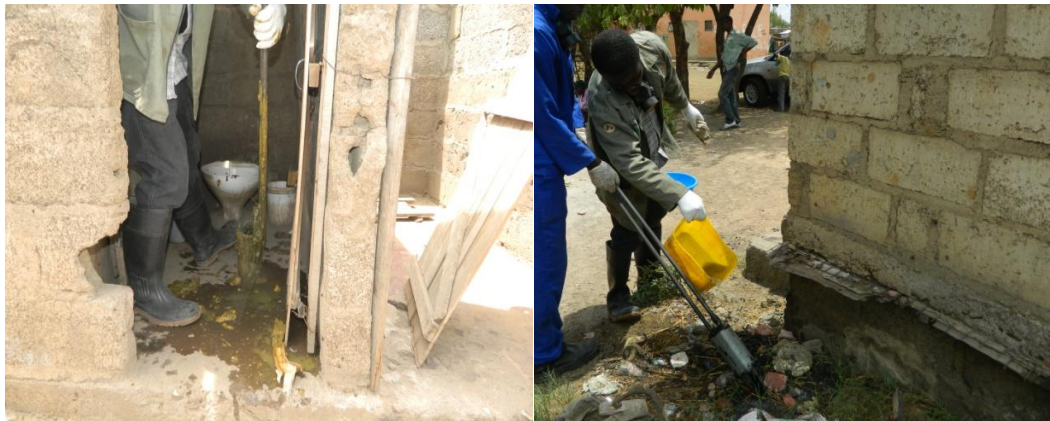
Figure 3-12: Faecal sludge sampling with the modified sampling tool (Source: This study)
