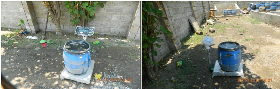
Figure 3-9: Weighing of the barrel together with the faecal sludge before separation (Source: This study)
