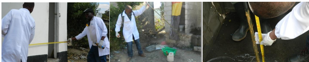
Figure 3-8: Latrine data collection (LHS: Measuring the dimensions of the pit latrine; Middle and RHS: Determination of faecal sludge depth in a latrine using a dipping rod).
