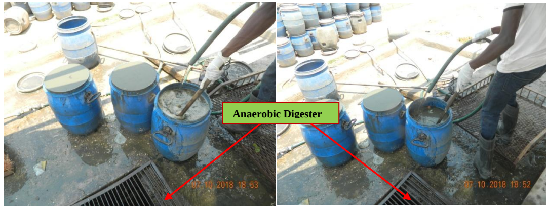
Figure 3-10: Washing of faecal sludge to separate the sludge from grit and solid waste (Source: This study)
