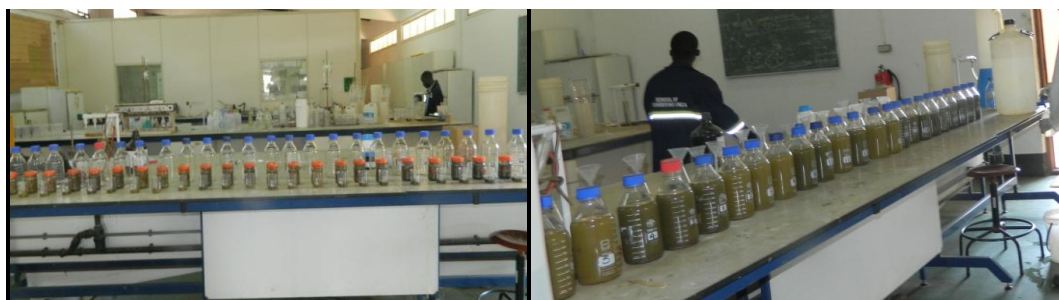
Figure 3-14 : Faecal sludge dilution (LHS: Faecal sludge in sampling containers before dilution; RHS: Diluted faecal sludge in 1 litre glass bottles) (Source: This study)
