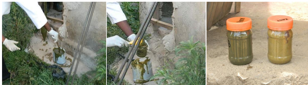
Figure 3-13: Faecal sludge sampling (LHS: Homogenisation of the sample in a 2.5 litre container; Middle: Transferring a homogenized sample into a labeled sampling container; RHS: Collected samples ready for transportation). (Source: This study)
