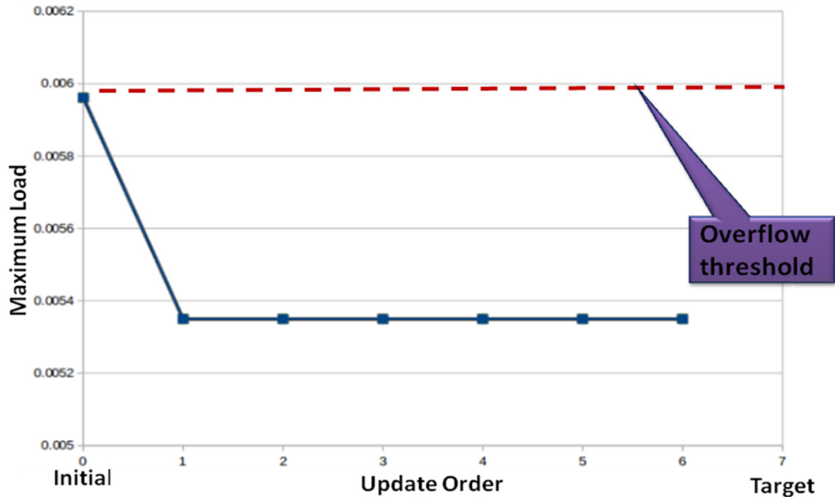
Figure 4.3.5: Traffic Isolation results for Voice Traffic _ Pan European Network
